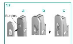
Center buttons of assembly with wall plate holes (17. a). When aligned, push buttons through holes and slide down to lock (17. b & c).
